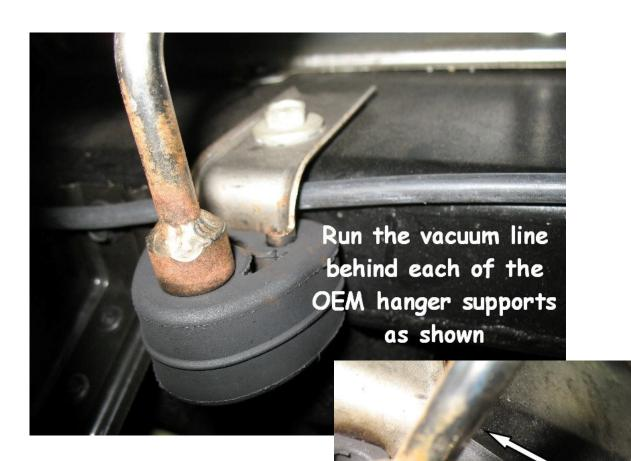
On the passenger side muffler hangers between the left and right hanger install the tee keeping the lines tucked behind the hangers
