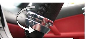
Grasp the chrome ring and rotate counterclockwise to unlock and pull down, **do not remove the boot from the ring unless you no longer want to use the chrome ring**
