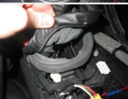
**5.** The plastic frame in question has two tabs at the ends of it's longer side. The tabs are held behind two small teeth. Use small screwdrivers to widen the teeth on one side and pull the tab up. You will notice the second tab will just slide away from the teeth that are holding it as you remove the boot.
