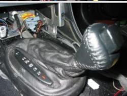
**4.** Remove the shift boot. Simply pull it off the frame by stretching the elastic. While doing so, you will notice the boot is still held down by the plastic frame which surrounds the gear display panel. Do not use force and do not pull on the boot just yet.
