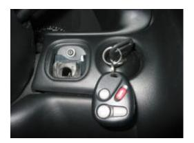
**10.** Remove the key from the ignition (if there's still one) and remove the center console. It will simply slide towards the rear of the car. Move it several inches first and remove the cigarette lighter connection that will be exposed now.
