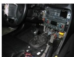
**3.** Remove the staple that holds the stock shift knob in place (bottom of the shift knob facing the front of the car). Remove the shift knob (simply pull it off).
