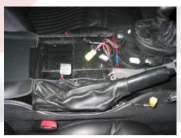
**12.** Install the new e-brake boot instead of the old one. Do not mind the metal frame embedded in the old boot, you will not need it and it will look just as good. If you do want to use the metal frame here is what to do...
