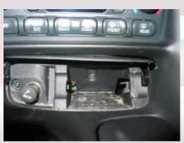
**8.** Remove the little trim piece next to the ignition key (pry it off with a small screwdriver from below).
