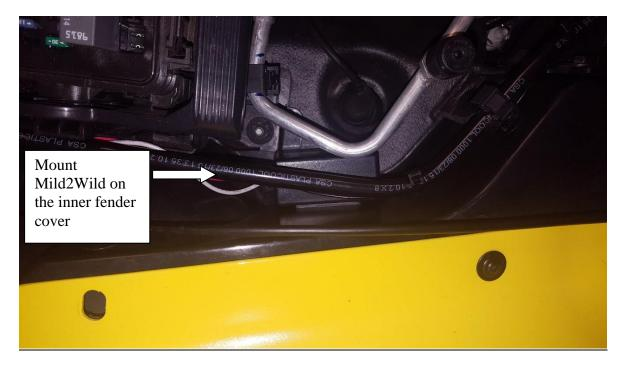
Attached the blue antenna wire as shown below and secure to the coolant line with the supplied zip tie
