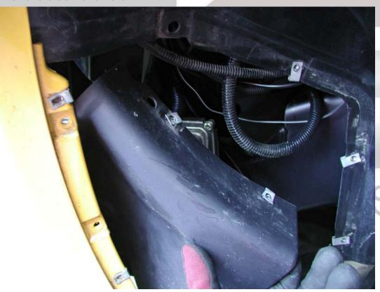
3. Both screens are the same for either side; please test fit the screens before taking the tape backing off so you are familiar with how they will be positioned. Use the provided alcohol pads to clear the inner fender surface were the screen will mount.
