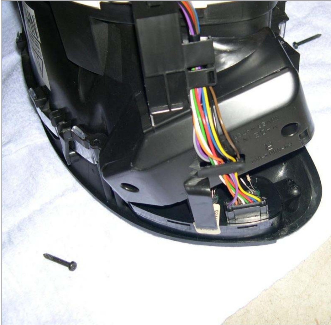
(27). This picture shows the face plate removed from the actual gauge cluster.
