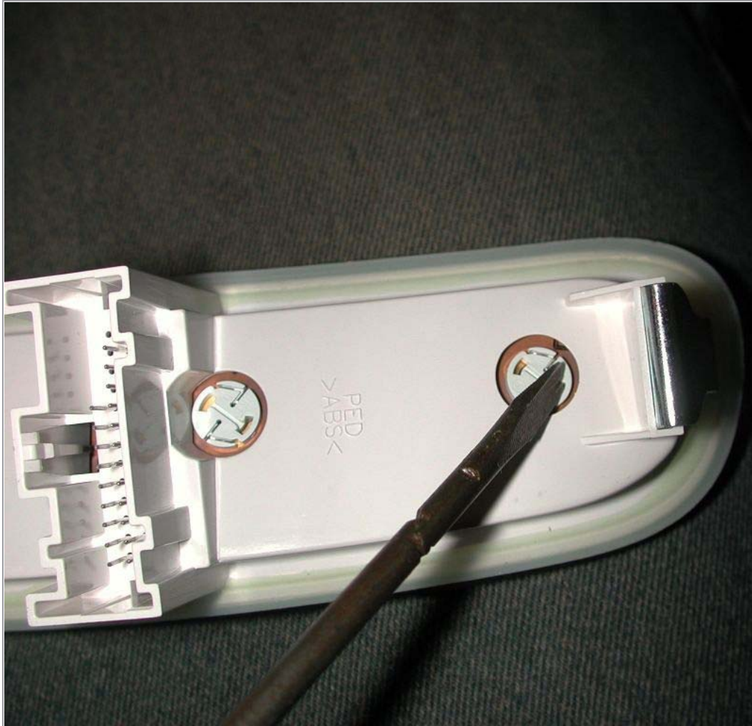
(30). One of the lights out of the panel. These guys are small .
