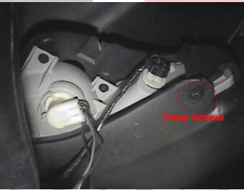
5) Remove the turn signal assembly. The Passenger side blackout is the one with the sticker on it.
