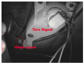
4) There is one more screw holding the turn signal in and that is 7mm. (off to the right of this picture but not seen now)
