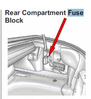
The rear compartment fuse block is located on the right side of the trunk behind a cover. Remove the convenience net retainers, the rear sill plate, and the passenger side trim retainers, then swing the trim out of the way.
