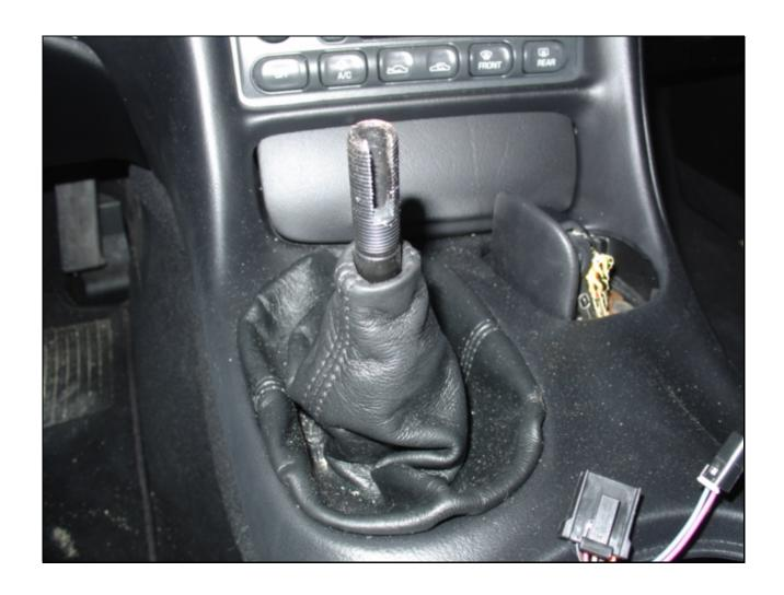
2) Now place your new C6 knob onto the shifter press down and turn clockwise until tight and in the correct location for you. Do not over tighten.
