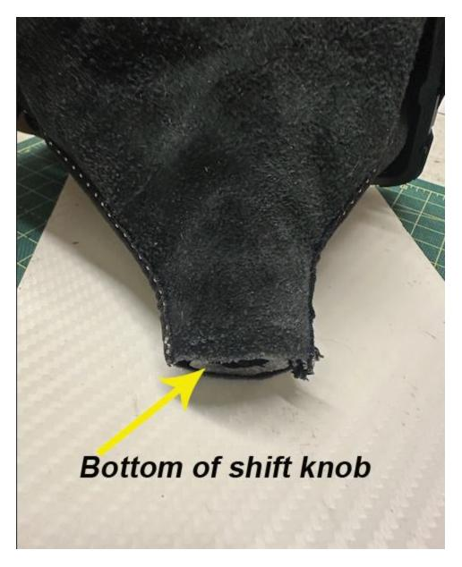
Take a zip tie or very tight rubber o-ring and place it around the boot resting inside the groove in the shift knob. This may be tough with thicker aftermarket leather boots so you can use a trim pry tool and work the leather first to create a
