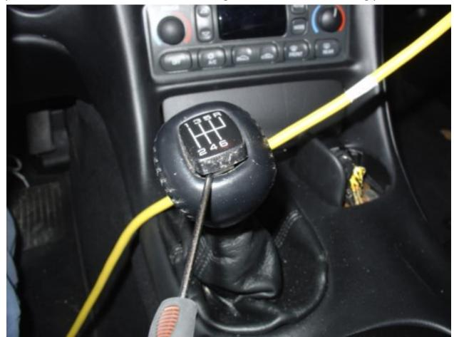
2) Using a pair of Vice Grips, grip the retaining pin tightly and pull the retainer pin up and out of the knob. You may have to rock the Vice Grips back and forth a little to get it all the way out. Just be careful not to damage anything else. We suggest that you cover the handle of the Vice Grip with a shop towel as the force when pulling up on this could cause you to hit the inside top of your Corvette.
