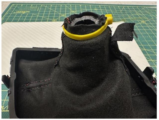
Now when you pull the boot down back into place in the console it will be attached to the knob and should look like this
