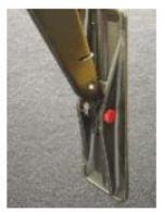
With a pair of Vise-grips, reach around your stock gas pedal and remove the retaining pin. It's a press fit so you may need to pull with some force to remove it. In some cases you may need to pry it out with a screwdriver or sharp wood chisel.
