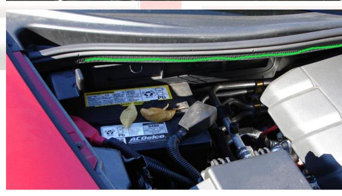
6) You can pull away the rear weather stripping to hide the wires if you would like (See below)
