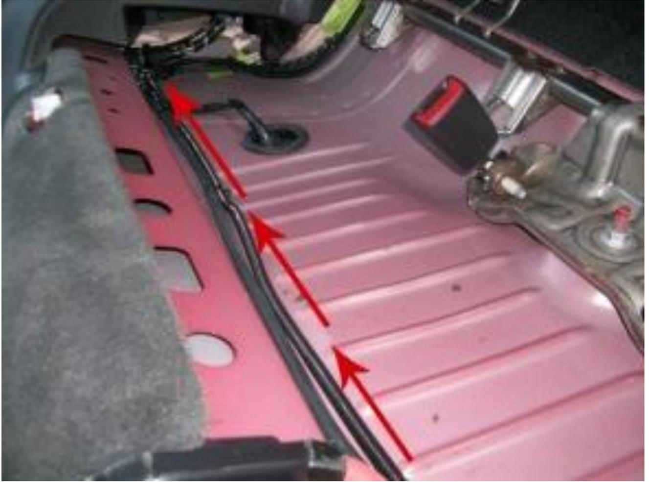
Once you get to the passenger side once you make the turn with the vacuum hose and power wire you'll be able to route and wire tie them to existing wires going around the turn and up over the seat back area. See photos below.
