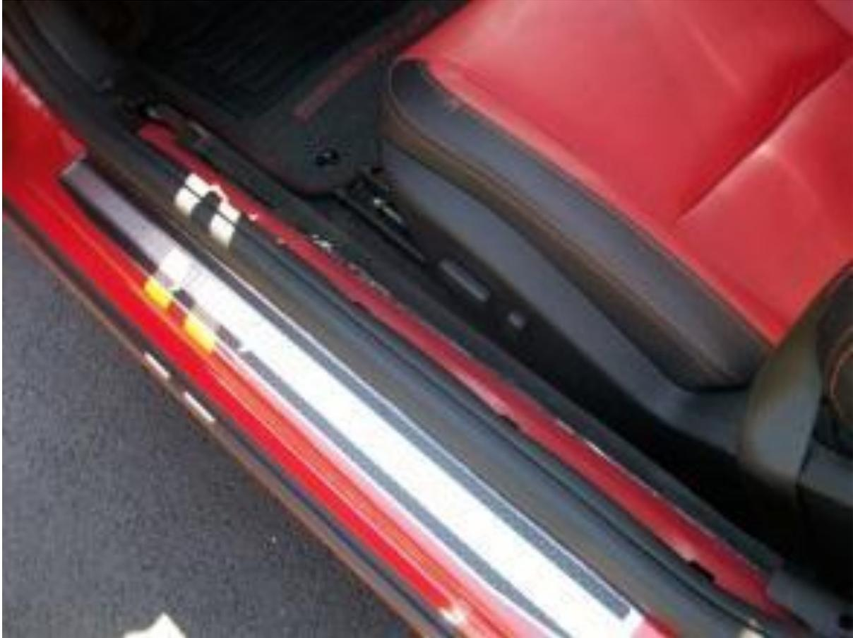
We now need to remove the driver's side kick panel. For this step you may want to remove the floor mat. When removing the kick panel the floor mat can get in the way. The sill trim plate had to be removed to remove the kick panel. In order to remove the kick panel you simply pull on each side to release the retainers and remove the panel out of
