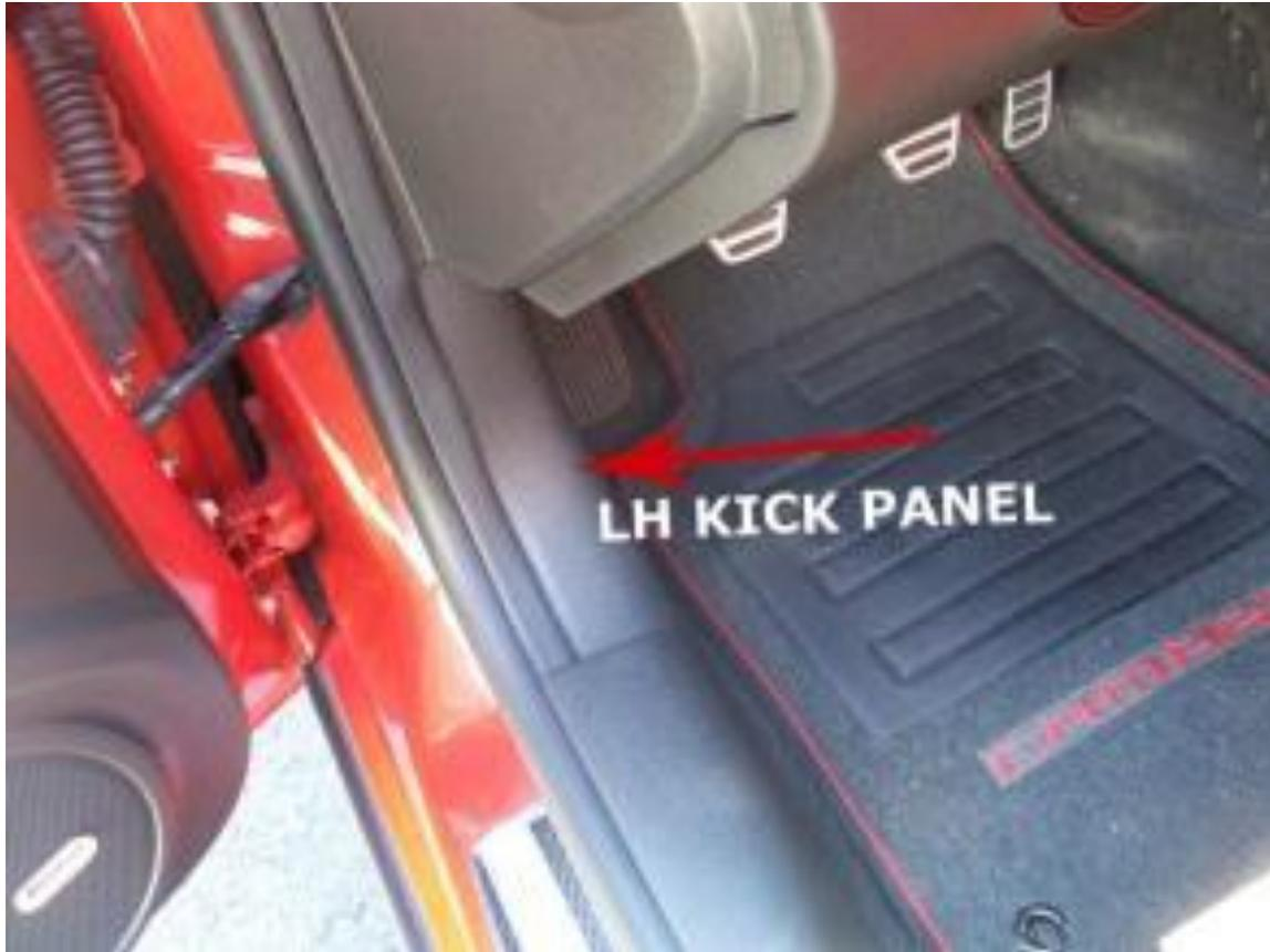
We will need to remove the driver's side sill trim plate in order to start. Simply pull up easily on each side of the sill trim plate to pop the retainers loose and remove the trim panel. See photo below.
