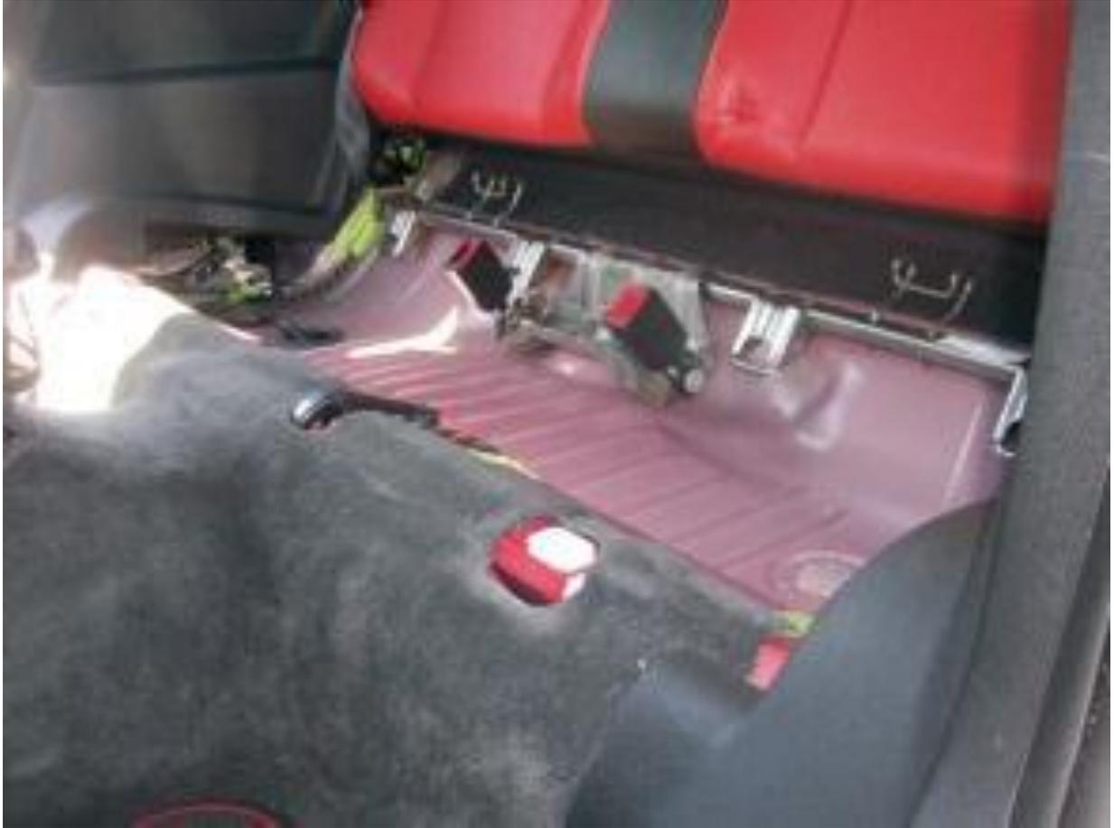
Once you reach the end of the runway, continue to run the hose and wire underneath the “B Pillar” or panel behind the driver’s head and door. See photo below.
