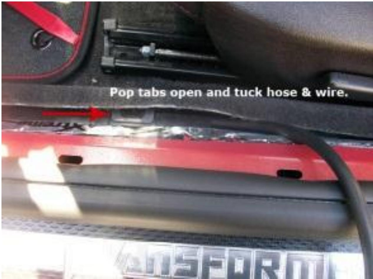
Remove the lower portion, or seat cushion of the rear back seat for the next step. In order to remove the seat there is a tab on each side of the front of the seat in the middle. Pop the tab and this will
