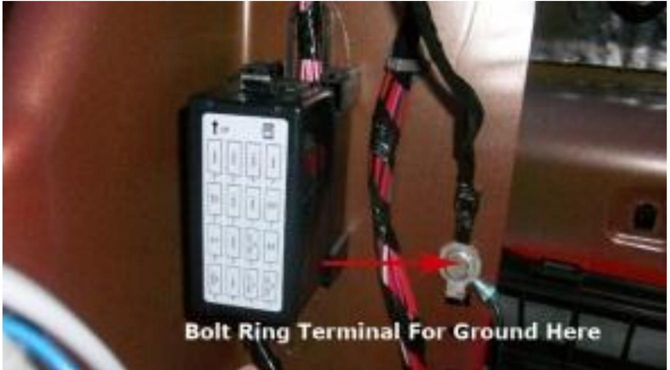
Since I had a custom sound application I custom mounted the NPP-In-A-Box in a hidden compartment behind an amp in my system. For stock applications I suggest using 3M tape or Velcro to adhere the NPP-In-A-Box to the area behind the passenger trunk carpet or doing some other type of configuration. Photo of mine mounted is below.
