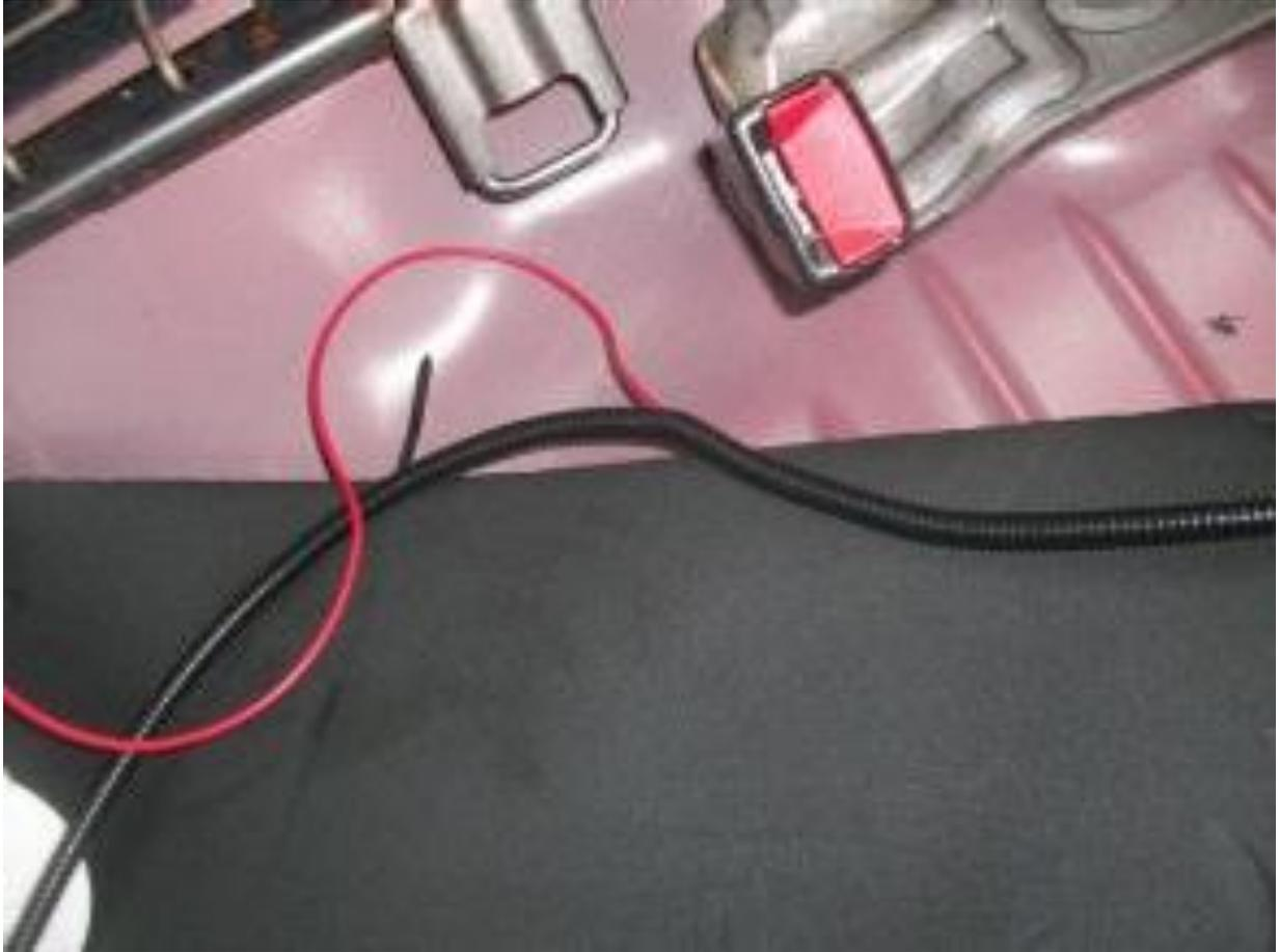
Once the loom is installed over enough wire you can start to run the vacuum hose and power wire across the rear seat cushion area all the way over to the passenger side. I used wire tires to tie the vacuum line and power wire to existing wires. See photos below.
