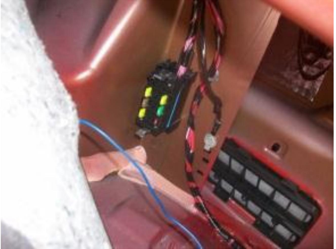
We are going to ground the NPP-In-A-Box to the bolt near the rear fuse block. At this point attach your ring terminal to the ground wire of the NPP-In-A-Box and unscrew the bolt near the rear fuse block and install the ground. See photos below.
