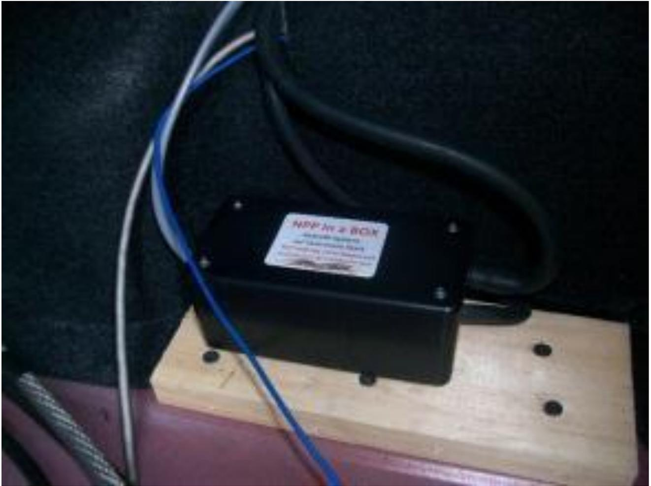
Once you have it mounted you can attach the power wire to the NPP-In-A-Box using a butt-connector, solder, etc. **The other end of your power wire will still not be connected to power and laying loose in the driver's side kick panel area.**
