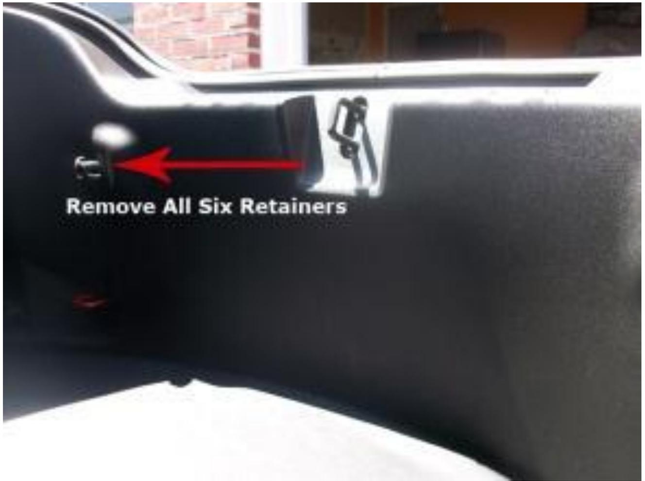
In order to remove the trim panel all you need to do is remove all six retainers. You would remove them by unscrewing them by hand. These would be the retainers used if you have a cargo net and if you don't that's where the cargo net would go.
