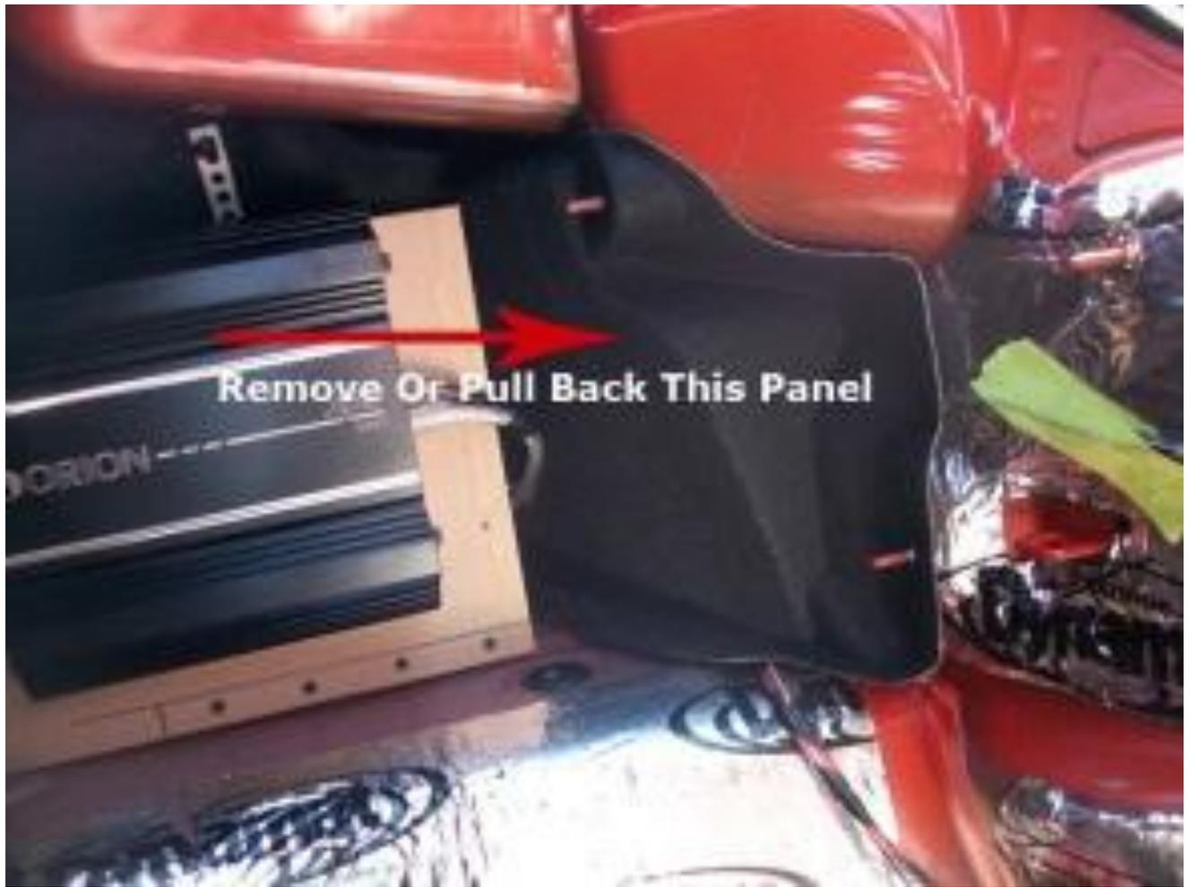
With the passenger's side trunk carpet panel removed or pulled back, you'll gain access to your vacuum hose and power wire for the NPP-In-A-Box. You'll also be able to see the rear fuse block. See photo below.
