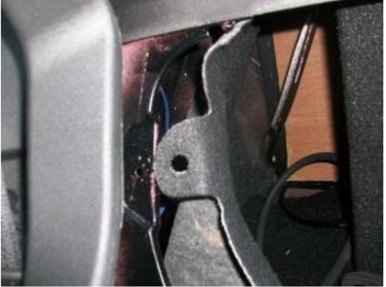
Once the retainer is removed you'll have access to behind the passenger's side carpeted trim panel in the trunk. For now, let the vacuum hose and power wire in that area. We'll come back to it in a step or two.
