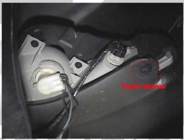
5) Remove the turn signal assembly.
