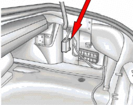
The rear compartment fuse block is located on the right side of the trunk behind a cover. Remove the convenience net retainers, the rear sill plate, and the passenger side trim retainers, then swing the trim out of the way.
