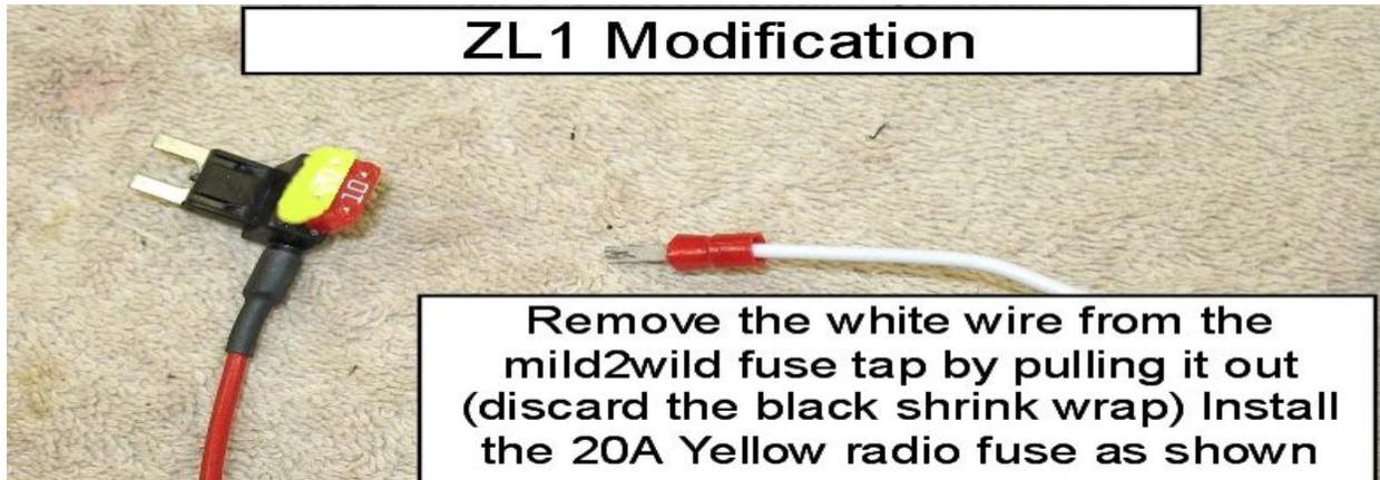
Complete the ZL1 modification above need to allow the use of the rear fuse box. Install the mild2wild fuse tap into the fuse position "F3" where you removed the yellow 20AMP, the red wire must be facing down as shown below. Take the white wire and install the red insulated blade connector into the **bottom slot** of the fuse position "F8" (where you removed the 10AMP exhaust fuse)
