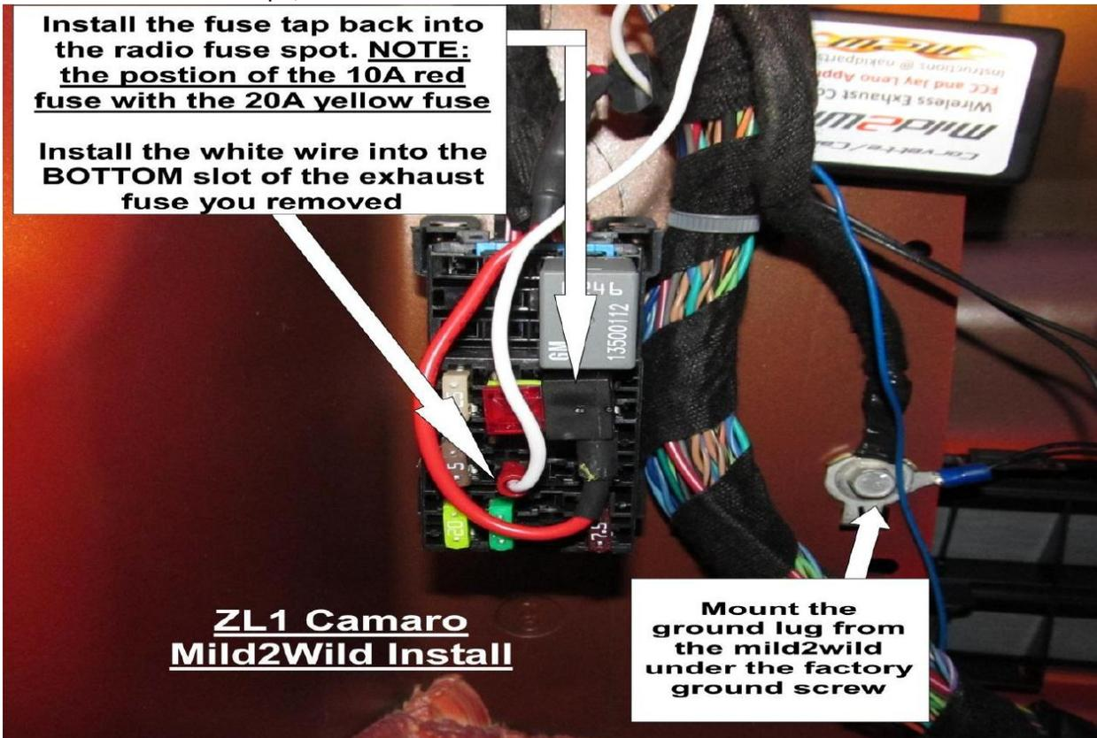
To reinstall the fuse box cover you will need to remove a small amount of the of material here to allow the wire to pass through. You can use a utility knife, file or dremel
