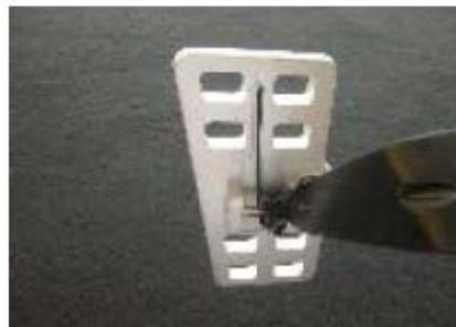
Once the spring is in the correct orientation, using the 3/32" Allen wrench and tighten the shoulder bolt.
