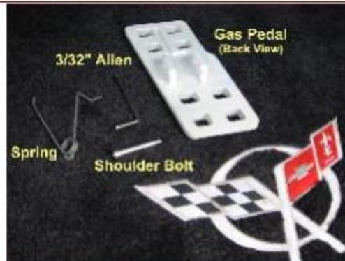
With a pair of pliers, reach around your stock gas pedal and remove the retaining pin. It's a press fit so you may need pull with some force to remove it.
