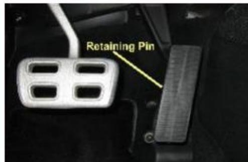
This is how the Gas Pedal Lever will look after the retaining pin has been removed.
