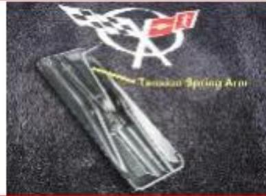
Next, insert the "supplied" 3/16" shoulder bolt into the Gas Pedal and begin to push it through the Gas Pedal Lever. Once the shoulder bolt has been started, install the Tension Spring Arm.
