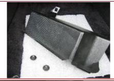
Next hold the aluminum Dead Pedal against the housing and mark the centers of each (2) screw hole. Leave no less than (2) ribs showing at the top to eliminate any interference problems with the screws.
